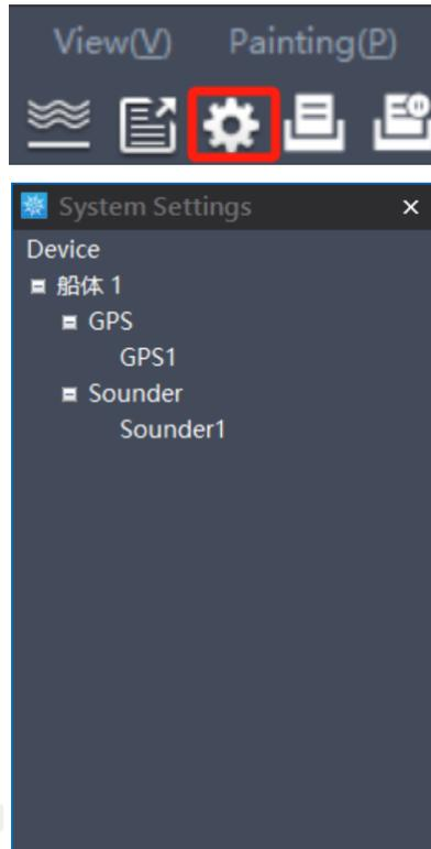
Double click "GPS 1" to enter the parameter setting interface of GPS device. Select the corresponding connection mode in "communication settings", enter "antenna coordinates", check "connection" in the lower left corner after setting, and click "OK" to complete GPS setting.
