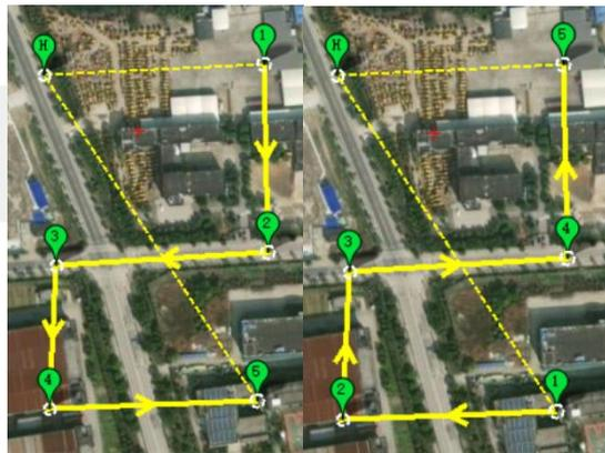
Loading/Overlaying KML: Right-click with the mouse to load KML. Select an existing KML or KMZ file to open and check the survey lines. Adjust them as needed and write them into the task points.
