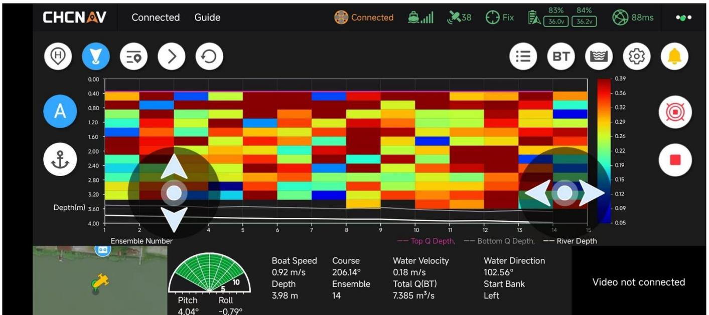
Flow velocity amplitude graph interface
