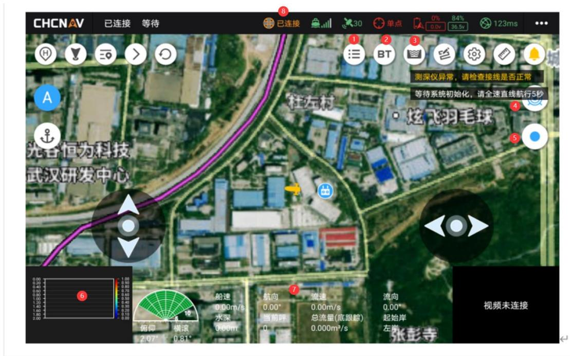
1. [Site Traffic Measurement Information]: Click this button to pop up the test task panel, where you can view the test task and the measurement information under the currently selected task, and you can create a new test task.
