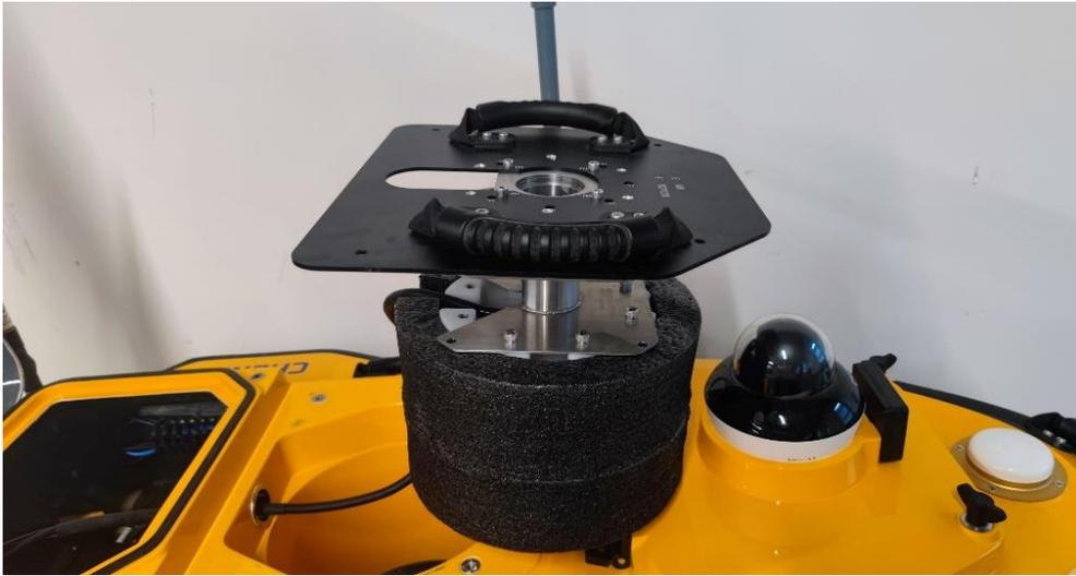
4. According to the ADCP model, find the mounting hole that is marked with the corresponding model on the mounting bracket, and connect the ADCP and the bracket tightly (the current bracket is a combined bracket, divided into three layers);
