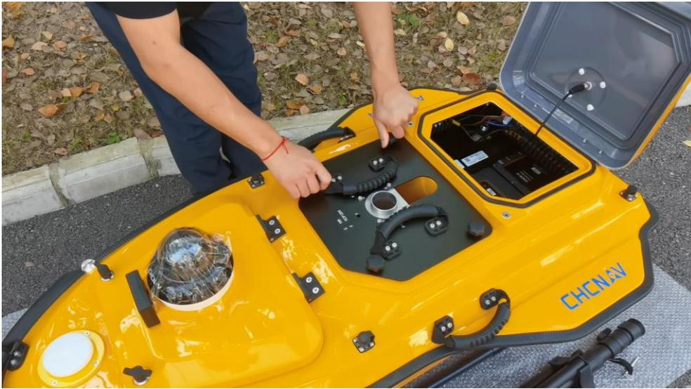
1. Open the rear hatch cover of the unmanned surface vessel, unscrew the 4 fastening screws on the black plate in the middle of the hull, remove the fixing plate, and remove the yellow protective cylinder in the middle of the hull, at this time the middle of the hull is connected up and down;
