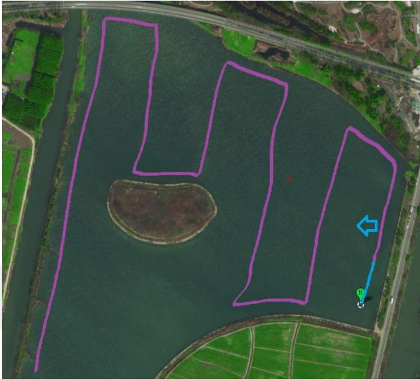
USVs automatically plan their routes in parallel directions, with millimeter wave and obstacle logic consistent with semi-automatic logic.
