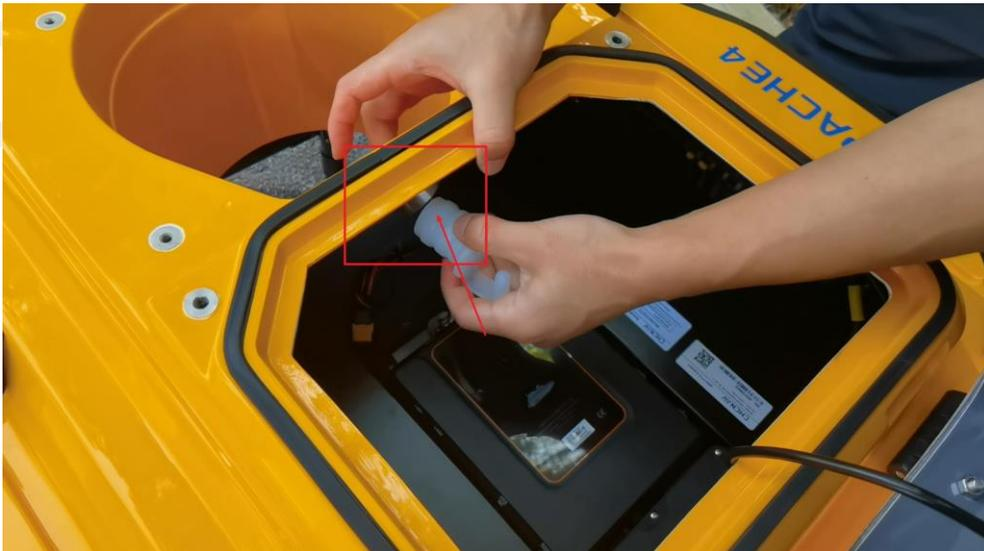
2. Remove the waterproof rubber plug from the inside of the aft cabin, and pass the cable through the reserved threading port from the cabin;
