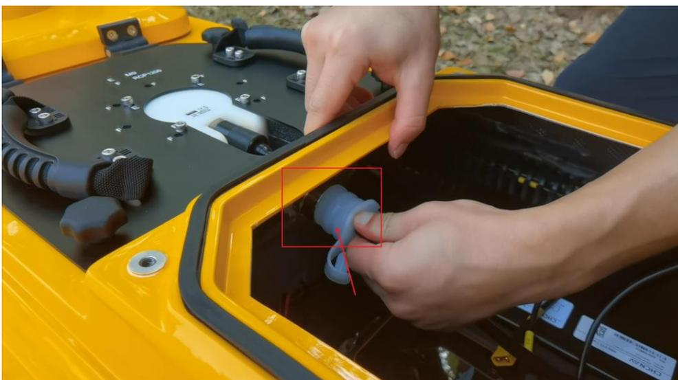
5. Assemble the bracket and fix the bracket to the boat, and at the same time, pay attention to the waterproof rubber plug after applying a certain amount of silicone grease;
